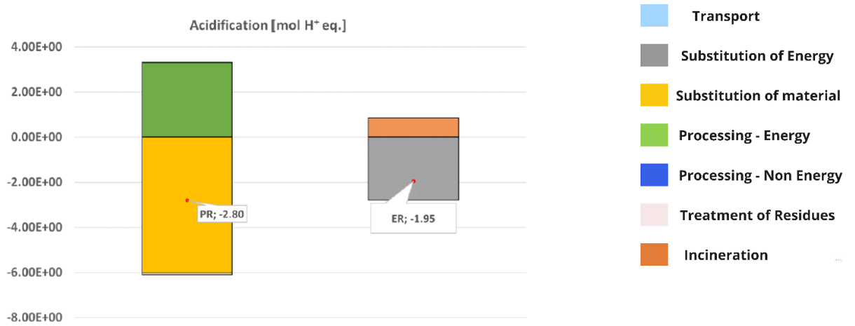
Figure 59: Comparison between physical recycling (PR) and incineration(ER) of 1 tonne of post-industrial PE/PA multilayer film waste – Acidification [4]
